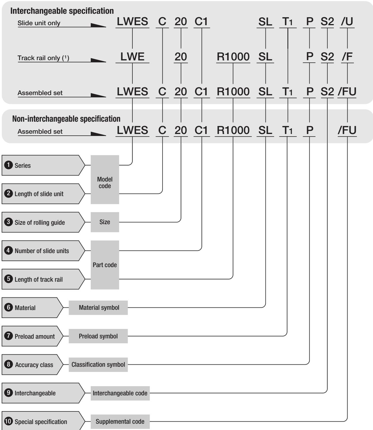
Note(1) : For the model code of a single track rail of interchangeable specification, indicate "LWE" regardless of the slide unit type to be combined.
