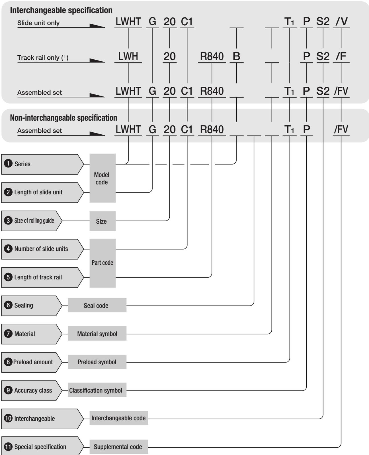
Note(1) : For the model code of a single track rail of interchangeable specification, indicate "LWH···B" (high carbon steel made) or "LWH···SL" (stainless steel made) regardless of the slide unit type to be combined.
