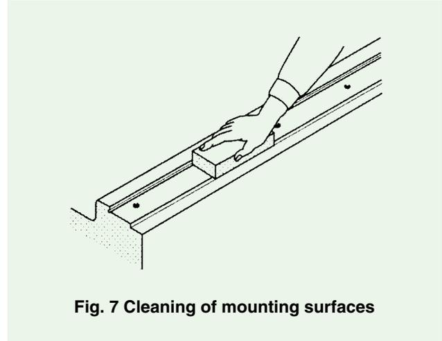
**Fig. 7 Cleaning of mounting surfaces**
