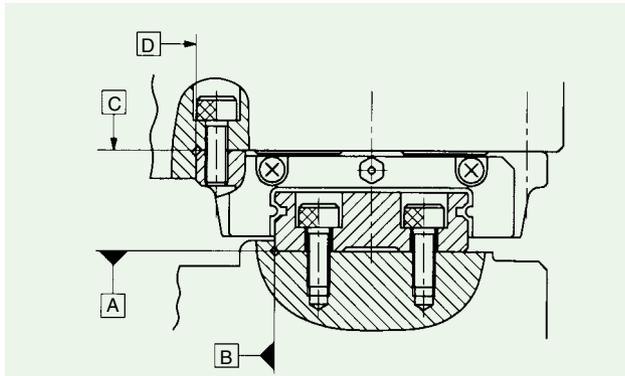
**Fig. 4 Reference mounting surfaces and general mounting structure**
