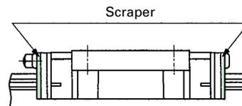
Metal scrapers are provided on the slide units of assembled set of interchangeable specification or non-interchangeable specification.
