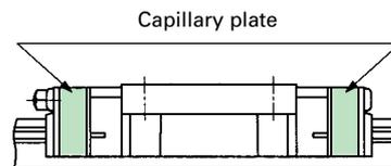
The capillary plate is assembled inside the end seal of the slide unit. It is impregnated with lubricant so that the re-lubrication interval can be made longer. For the total length of the slide unit with capillary plates, see Table 7.
