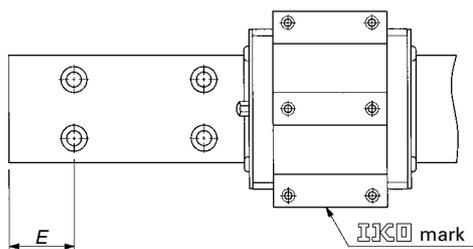
The mounting hole positions of track rail can be specified by specifying dimension E at the left end, which is the distance from the mounting hole nearest to the left end of the track rail to the left end face of the track rail in sight of mark on the slide unit. When ordering, add the dimension (in mm) after "/E". Dimension E can be specified in a limited range. Consult for further information.
