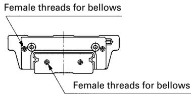
For an assembled set of interchangeable or non-interchangeable specification, female threads for mounting bellows are provided on the slide unit and the track rail. For details of related dimensions, see Table 6.
