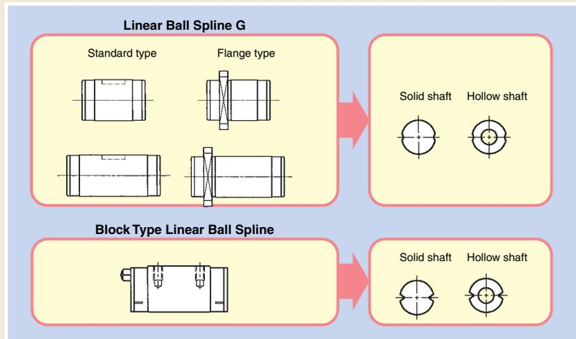
The raceway structure of spline shaft of Linear Ball Spline G and that of Block type Linear Ball Spline are different. So, the spline shafts of these two are not interchangeable.
