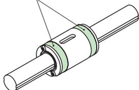
The standard synthetic resin end caps are replaced with stainless steel end caps, keeping the total length of the external cylinder unchanged.
