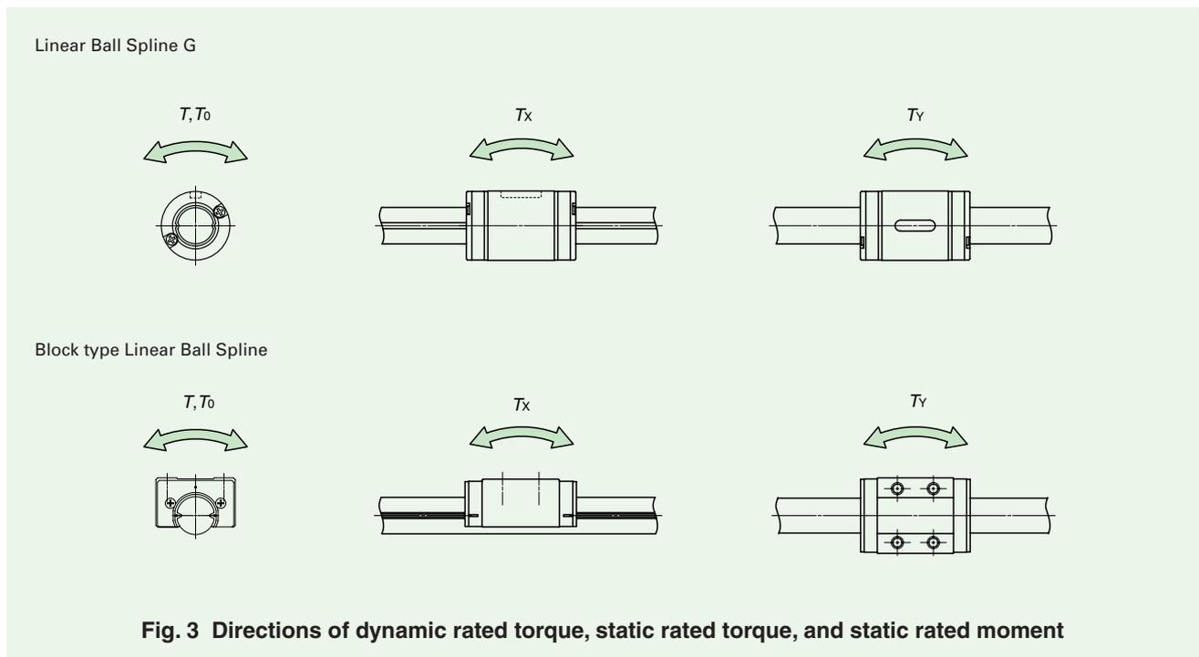
**Fig. 3** Directions of dynamic rated torque, static rated torque, and static rated moment
