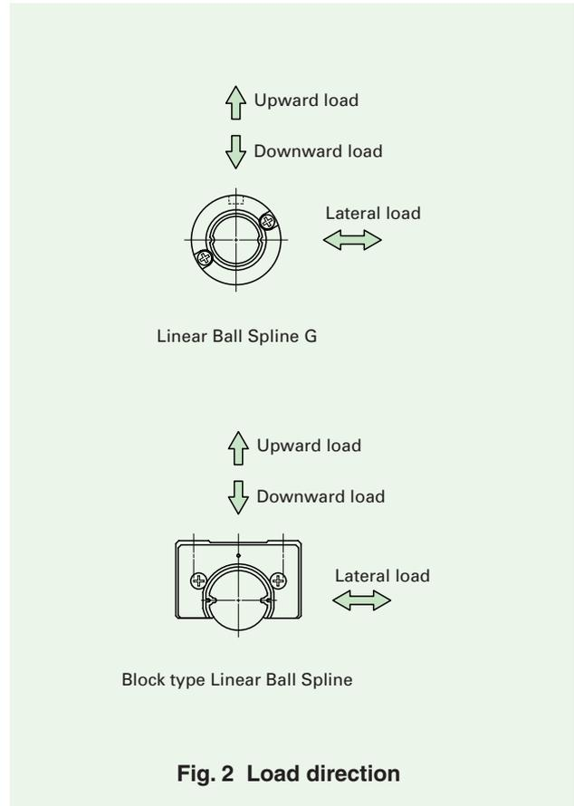
receiving the maximum load when a torque or moment (See Fig. 3.) is loaded. They are the allowable limit torque or moment that permits normal rolling motion. Generally, they are used in combination with the static safety factor.
