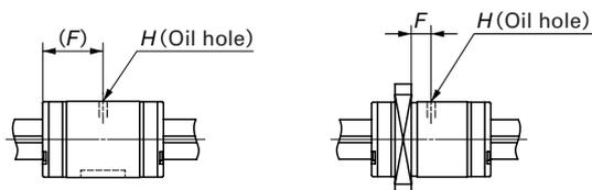
An oil hole is provided on the external cylinder of Linear Ball Spline G. For details of dimensions, see Table 9 and Table 10.
