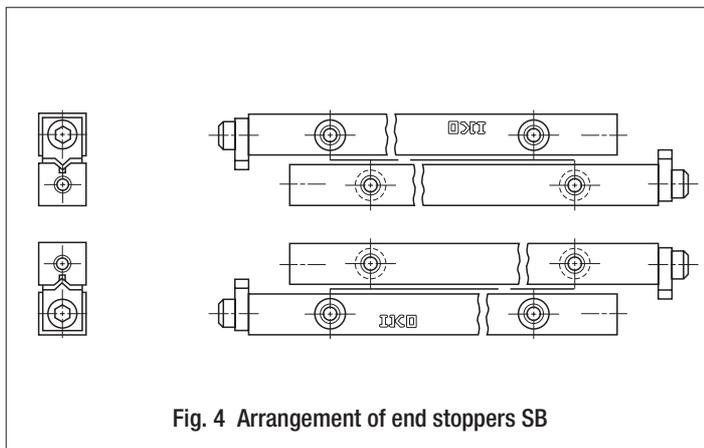
Fig. 4 Arrangement of end stoppers SB
