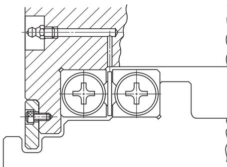
Fig. 6 Example of lubrication method
