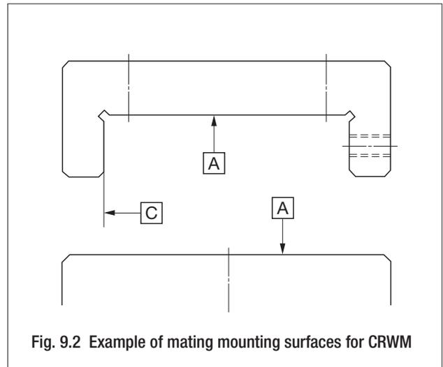
Fig. 9.2 Example of mating mounting surfaces for CRWM
