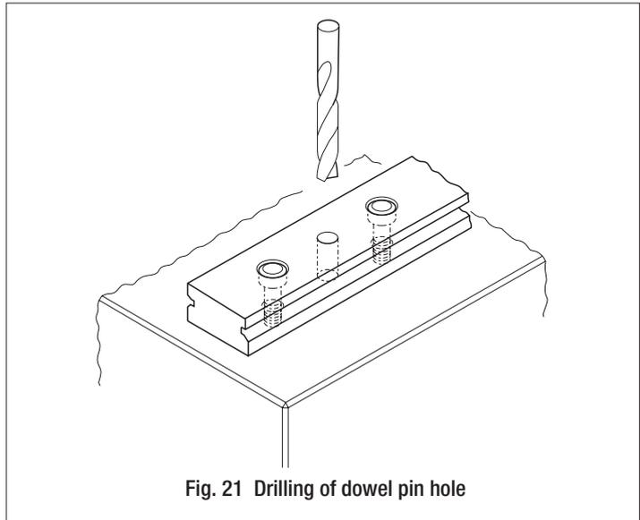
Fig. 21 Drilling of dowel pin hole
