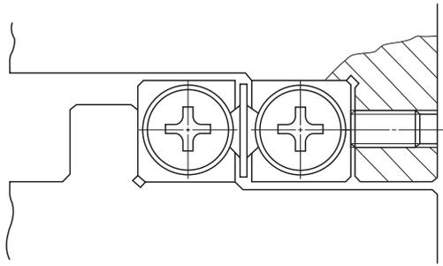
Fig. 10 General example of preload
