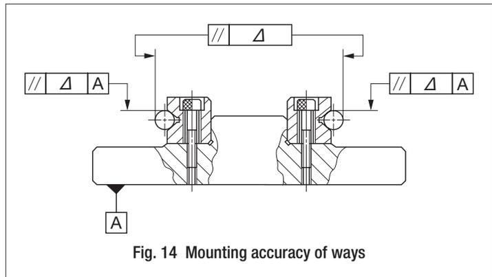
Fig. 14 Mounting accuracy of ways
