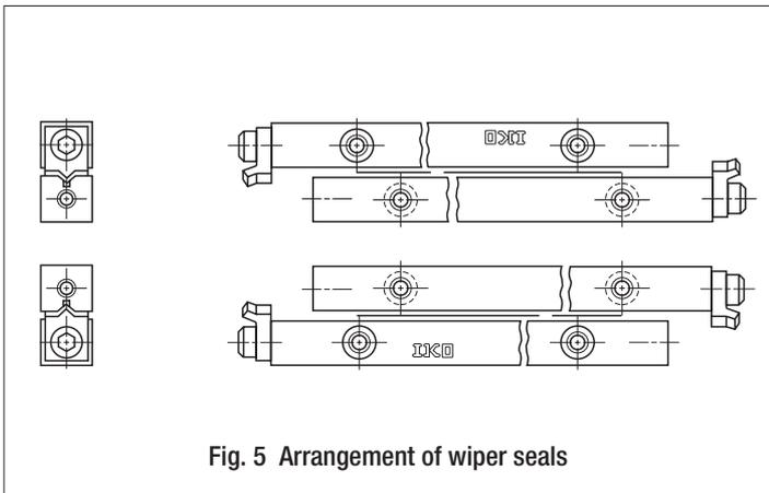
Fig. 5 Arrangement of wiper seals
