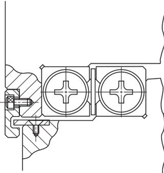
Fig. 7 Example of non-contact type shield (Labyrinth seal)
