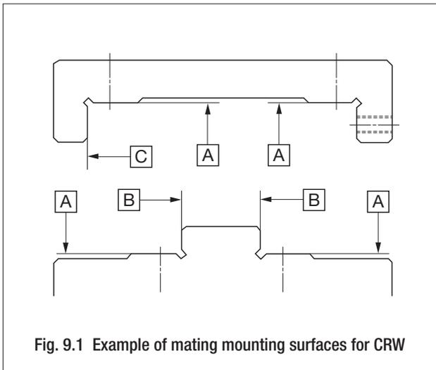
Fig. 9.1 Example of mating mounting surfaces for CRW
