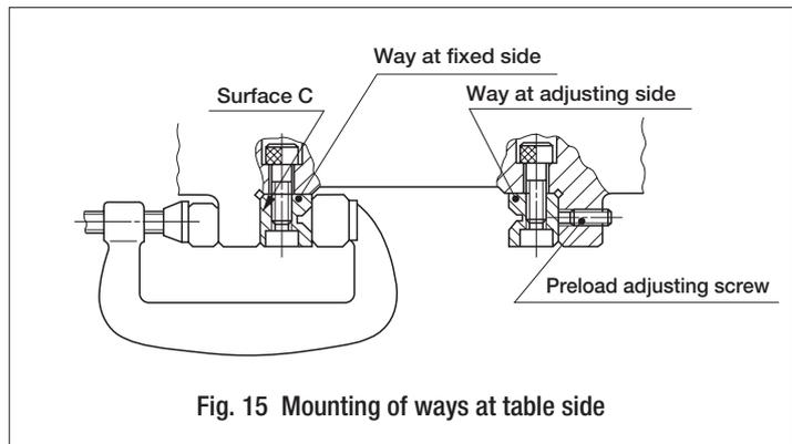
Fig. 15 Mounting of ways at table side
