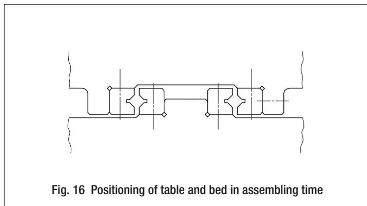
Fig. 16 Positioning of table and bed in assembling time
