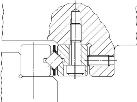
Fig. 2 Mounting example with special mounting screw
