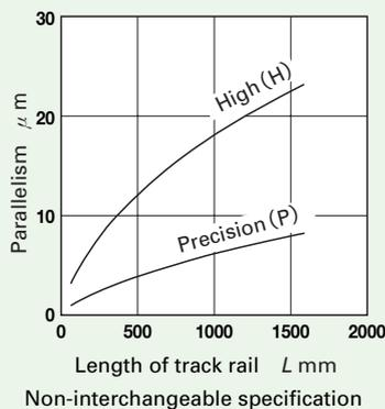
**Fig.1 Parallelism in operation**
