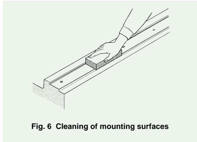
**Fig. 6 Cleaning of mounting surfaces**
