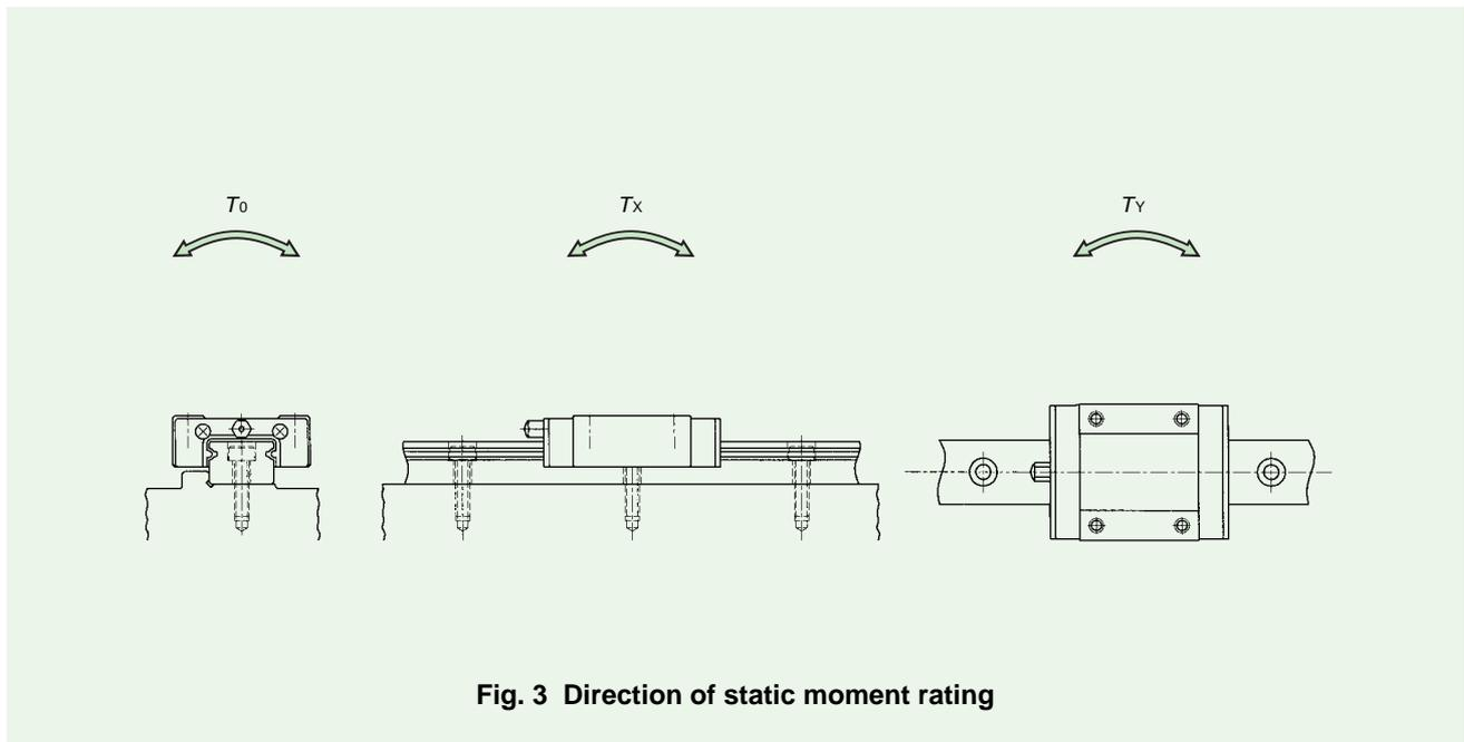
Fig. 3 Direction of static moment rating
