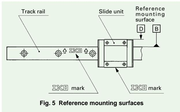
Fig. 5 Reference mounting surfaces
